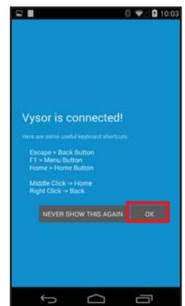
The Android’s screen should be mirrored on the PC’s monitor. Interaction with the Android device can now occur on the device itself or via the PC interface (i.e. keyboard, mouse). Once mirroring is complete, continue choosing audio connection method.
