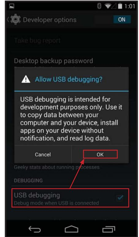
Connect the Android device to the computer via the USB slave or OTG port. ADB drivers should then be installed. If they are not installed automatically, do a Google™ search for the appropriate drivers and install them (example: for a Google Nexus™ 5 device, search for “Google nexus 5 ADB driver”). If product-specific ADB drivers cannot be found, install “Generic” ADB drivers (also can be found via web search, or within the application interface shown later).
